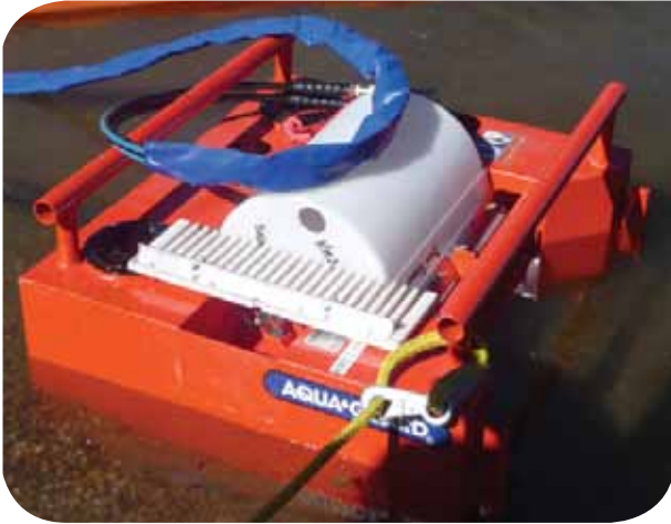
Skimmers are used on concentrated quantities of pooled oil
