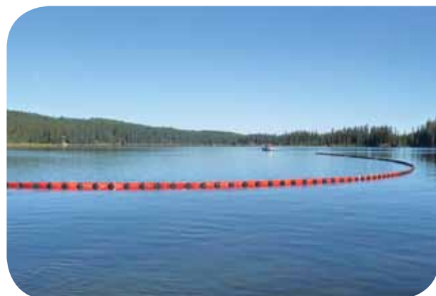
Deflection boom diverts oil away from the sensitive area to a less sensitive location for recovery
