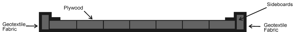
Bridge Travel Surface Profile View (Not to Scale)
